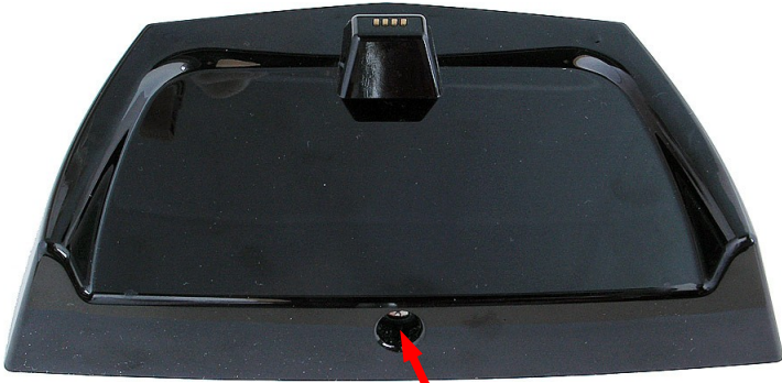
Power Supply 12Vdc
