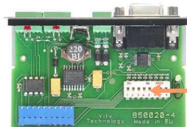
Dipswitches to setup the address
