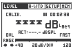
Fig 3.4 SPL Panel with Overload
