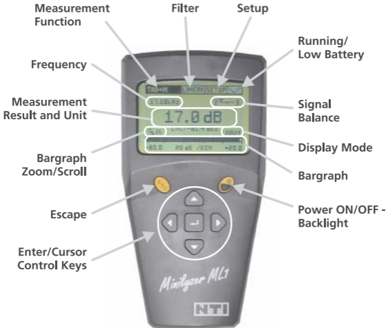
Fig 2.1 Display & Control Elements
